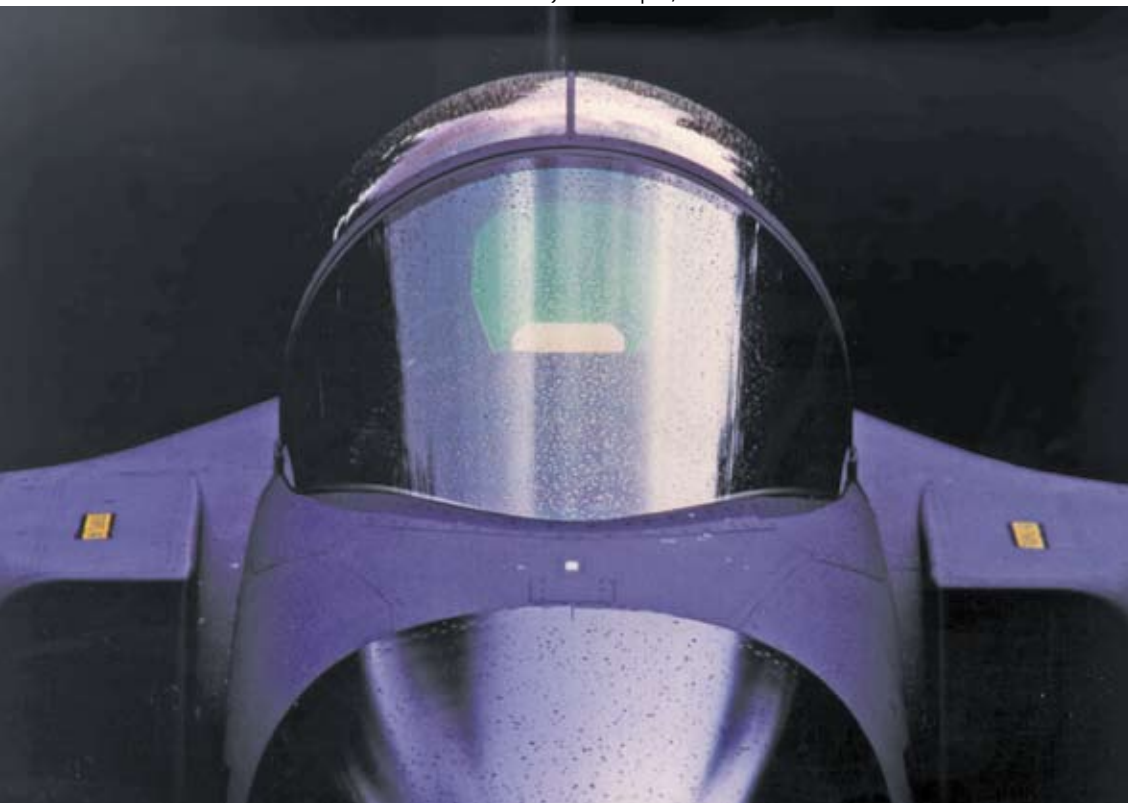
JAS 39 Gripen, windshield made from PLEXIGLAS® GS 249 Stretched
